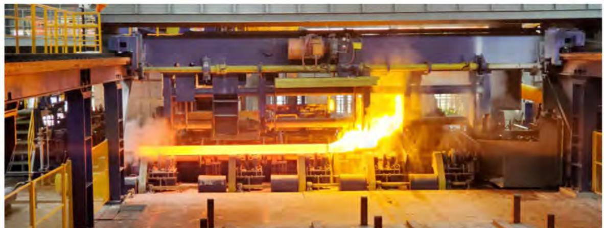
A piece of hollow bloom being processed (nitrogen blowing and borax blasting) before entering the downstream mandrel pipe mill
