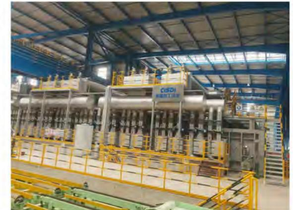
Reheating furnace for 1,500mm hot strip rolling line
