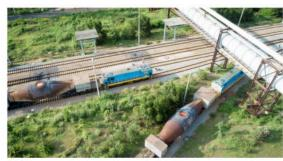
CISDI's autonomous locomotive, loaded with hot metal, traverses the railway crossing from ironmaking plant to steelmaking at Zhanjiang Steel
