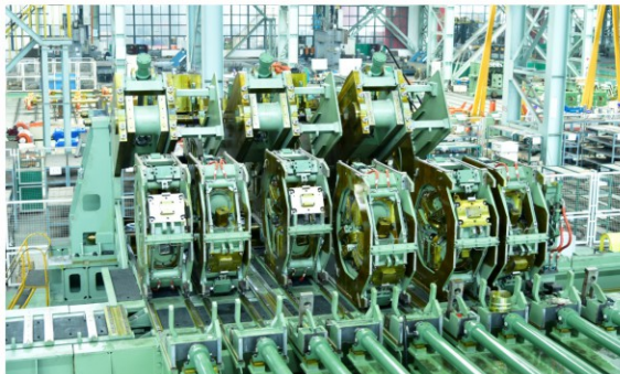
The tube mandrel mill being manufactured and assembled in the workshops at CISDI Equipment Co. Chongqing
