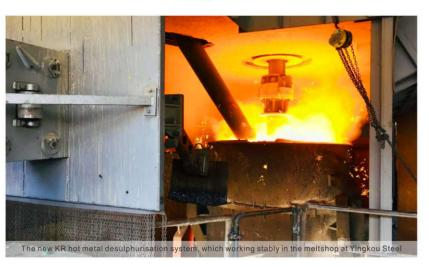
A new KR desulphurisation system has been successfully hot-commissioned at the steelmaking shop in Yingkou Steel, Northern China.
