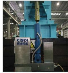
CISDI's new servo oscillator for caster mould at SFRE
