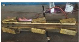
Wedges with deposit welding completed by the robot
