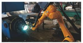
The rotary arm of a deposit welding robot in action
