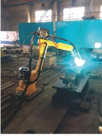
The working plane of a deposit welding robot
